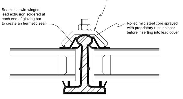
No.7 'Heritage' Lead Covered Steel Glazing Bar with 28mm Double Glazing infill
